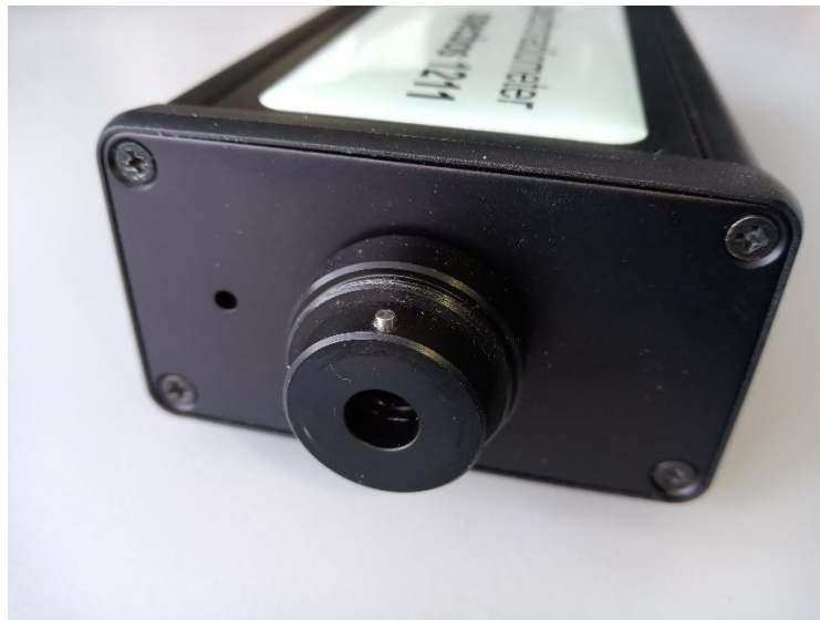
Front face of specbos 1211-2 with hole for sync detector (left of the measuring head)
