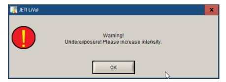
Adjust the intensity by decreasing or increasing the measuring distance. Regardless of underexposure the measurement is valid. In case of overexposure the results are not valid and will not be shown.
