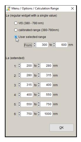
For the regular 1-value Le widget, there is a choice between the wavelength range that corresponds to the visible light (380 nm to 780 nm), the entire calibrated wavelength range (specbos 1201, spectraval 1501 and spectraval 1511: 380 nm to 780 nm; specbos 1211: 350 nm to 1000 nm; specbos 1211 UV: 230 nm to 1000 nm) and user selected range.
