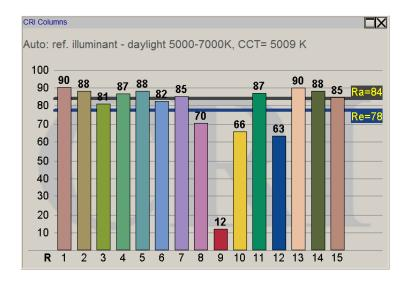
The widget displays the CRI data in columns.  $R_a$  and  $R_e$  indices are shown as two lines in the background.
