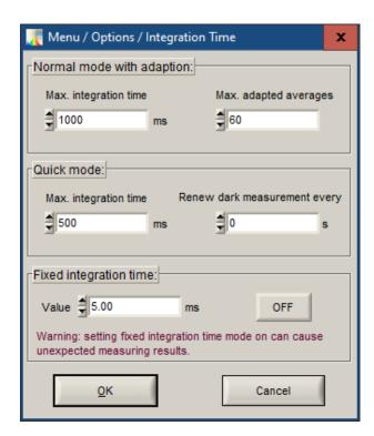
'Max. integration time' and 'Max. adapted averages' (**spectraval** only, for other devices this control is not visible) are internal device parameters which have influence on the behavior of the integration time adaption algorithm. The setting is saved to the internal
