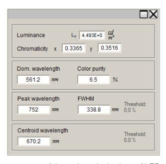
The widget displays a summary of the main optical values of LEDs.
