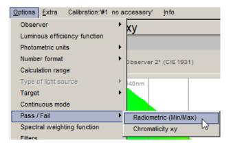
The radiometric quantities are characterized by a value and a tolerance (relative or absolute alternatively). The tolerance of xy can be characterized by a polygon with 3 to 15 vertices or by the McAdam ellipse.
