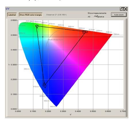
The color coordinate diagram contains the Planckian curvature for orientation. The actual measuring values are indicated in the diagram.
