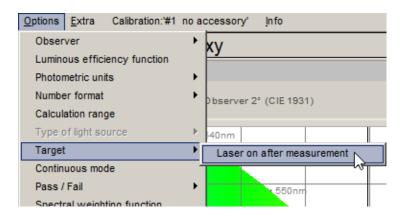
The Options Target Laser on after measurement causes the target laser to be switched on again automatically after a measurement. This feature can be used for a new adjustment of the measuring area.
