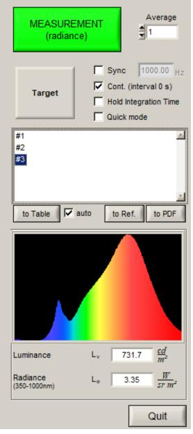
The measurement procedure consists of a first spectra acquisition using a fixed integration time, a subsequent calculation of the best integration time for a well-driven spectrum, a second measurement with this time and a final dark spectrum measurement. In some cases, more adaptation steps are necessary. You will be informed about the status of the measurement on the edge of the screen below the diagram: 'Adaption to exposure' or 'Performing measurement'.
