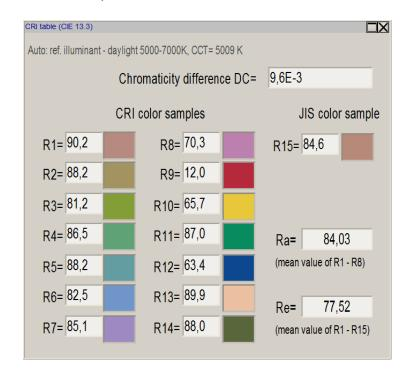
The widget displays all CRI-relevant numeric results with color samples for better orientation. Additionally, the chromaticity difference DC between the test object and the reference illuminant is shown.
