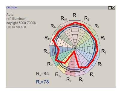
The widget displays the CRI data as a circle diagram.  $R_a$  and  $R_e$  indices are shown as two thin circle lines in the background.
