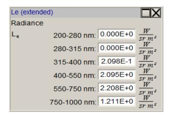
Shows 6 radiometric values calculated in specified wavelength ranges. Depending on the used accessory the values have a meaning of Radiance, Irradiance, Radiant Flux or Radiant Intensity.
