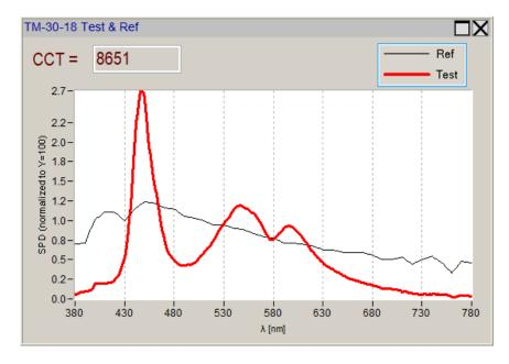
The widget displays Correlated Color Temperature, the measured spectrum and generated on the basis of CCT reference spectrum, which is either daylight or Planckian standard illuminant, or a mixture of both (as native IES TM-30-18 calculation tool does).
